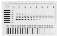
CW02 Crack Width Ruler
